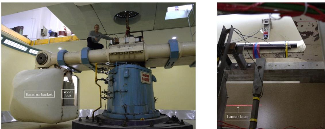
(a) Geotechnical centrifuge at the IWHR
